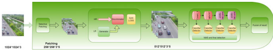
Fig. 2 SR-OIR-SSD combine four-block selective patching, GAN, object detector, and fusion of results. RGB image of size (1024 \times 1024 \times 3) feeds to patching block, which converts it into multiple patches of size (256 \times 256 \times 3) with an overlap of 128. Selective patching only generates patches containing objects. All these patches feed to GAN, increasing its resolution by two with high PSNR. The output of the GAN feeds to the object detector to perform detection. In the end, output of all the patches combines for the final result
